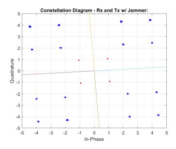
It is noted that the received signal is demodulated to exactly the jammer message (The 'jammer bit error rate' is zero). This is expected, given that the jammer signal is modulated identically, whilst being considerably more powerful.
