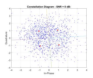
Case 4 : SNR = 0dBTotal number of its in error: 385 Obtained BER: 0.160 (to 3 s.f.)
