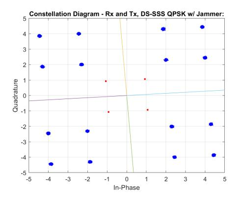
The SSS is incredibly effective, with the BER = 0. The modulation scheme is also very effective at reducing the impact of the noise, with the BER equal to 0 when the SNR = 0dB. Sacrificing the BUE has resulted in the a system that is considerably more robust to both noise and a jammer.
