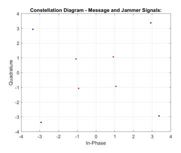
The constellation diagram for the received signal is shown below (red denoting Tx and blue denoting Rx):
